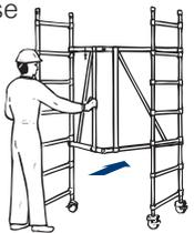
**3** Insert deck on 2nd rung of tower.
