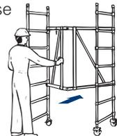
**3** Insert deck on 2nd rung of the tower.
